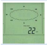
The wind speed unit can be set to read in mph (miles per hour), km/h (kilometers per hour), bft (Beaufort), knots or m/s (meters per second). The default unit is mph.
